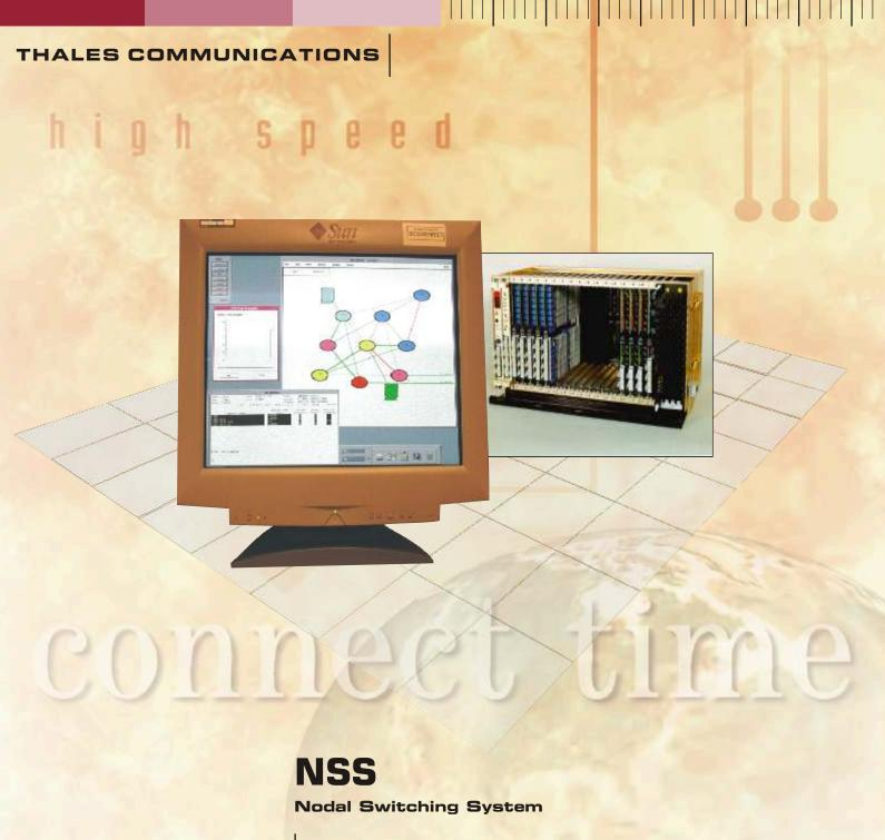
The building block of the NSS is the NSU - Nodal Switching Unit. The NSU is a small-size modular ISDN digital switch ideally suited for military applications. Any number of NSUs can be interconnected to form networks of any size. Its unique networking capabilities ensures network transparent features and free numbering scheme.
